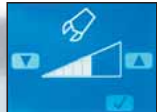
Fine tune hydraulic flow adjustment screen in A (active) or E (economy) mode
