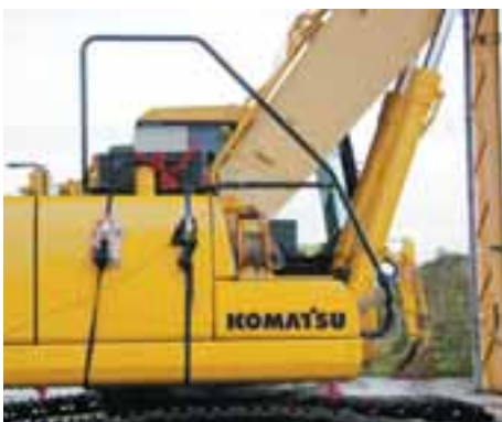
PC340 demolition machine, carrying test instrumentation.
