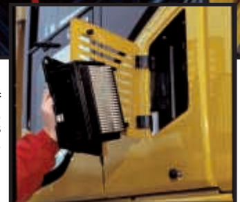
Easy removal/installation of air conditioner filter element, without tools facilitates easier cleaning.
