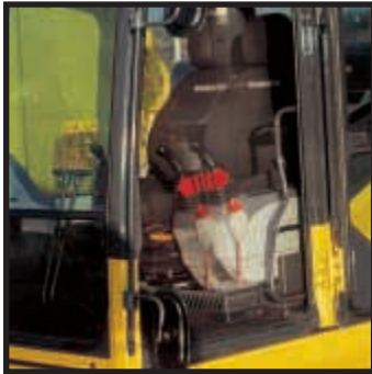
Seat sliding range: 340 mm - increased by 120 mm compared to dash 6 machines
