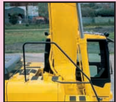
Large handrail for safe access
