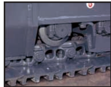
Track Link with Strut The PC160LC-7 uses track links with strut, providing superb durability.
