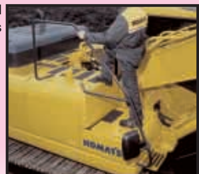
Large handrail for safe access
