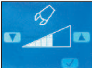
Hydraulic flow fine adjustment screen in A (Active) or E (economy) mode.
