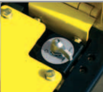
Battery Master Switch
