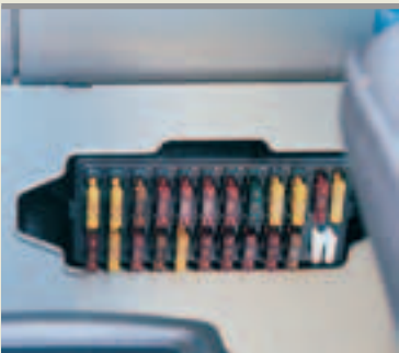
Centralized Fuse Box
